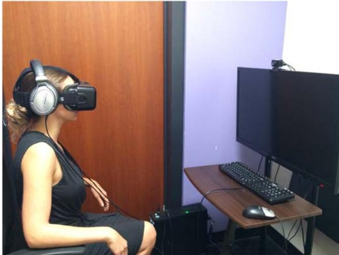
**Figure 1.** Participants were placed in a fully immersive virtual environment with the setup illustrated above. They donned a head-mounted display (HMD) through which they were able to view the stimulus. Sensing equipment tracked users' head motion so that a realistic visual depiction of the environment could be updated constantly based on the direction of the participant's view. The accompanying acoustic track was played through headphones, as pictured.
