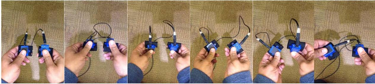
**Figure 3.** The positions of the orientation trackers on the fingers, in various configurations, attached with custom Velcro™ straps. (a) The initial default positions; (b) Both pitched down; (c) Both pitched up; (d) Both yaw'd; (e) Right pitched up, left yaw'd; (f) Right pitched down, left yaw'd.
