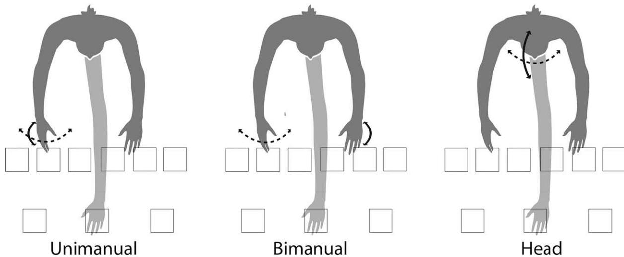
**Figure 1.** A top-down view of our three control schemas. The dotted line of the controlling appendage maps to the third arm yaw (rotation about the vertical axis), while the solid line maps to the third arm pitch (rotation about the horizontal axis running from left to right).
