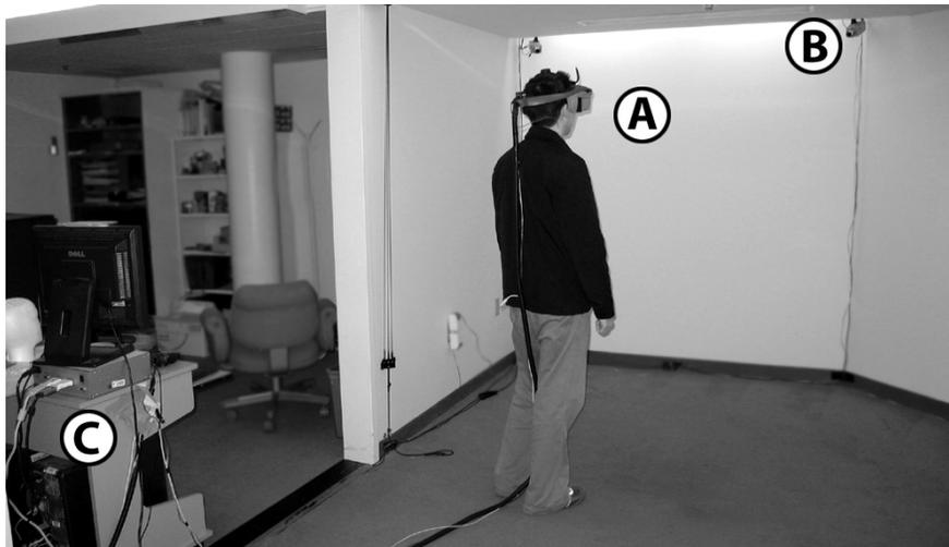
**Figure 2.** Equipment setup: A) head-mounted display and orientation tracker, B) positional tracking camera, C) rendering machine.
